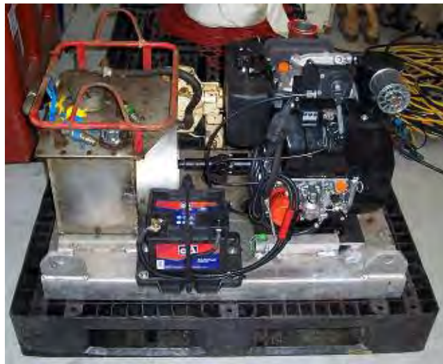
GAMBAS® 50 Back Deck Equipment – Mini hydraulic plant for the stop-and-go winch
