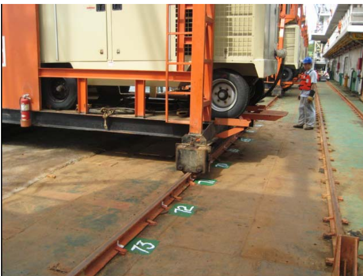
Marks along the rail of the drill rig.
