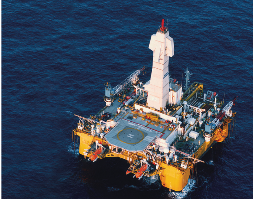
The Henry Goodrich semi-submersible oil rig operating in the waters off Newfoundland and Labrador.
