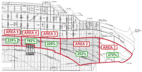
Figure 8. Relative strength of MV Qajaq W over MV Apollo
