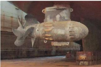
Figure 1. Propeller and thruster of MV Qajaq W.
