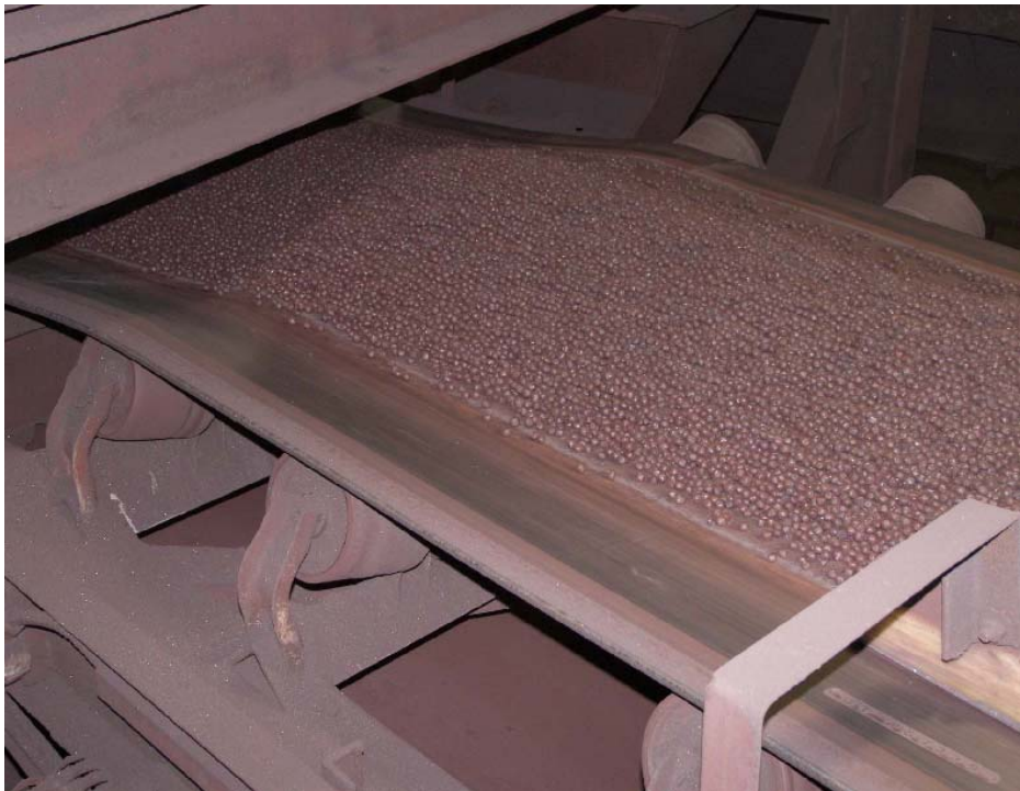
Photo: Iron ore pellets move along a conveyer at IOC's operation in Labrador City
